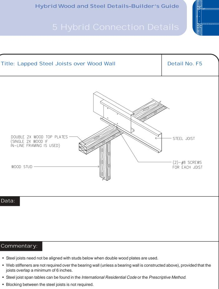
• 10d nail can be used in lieu of #8 screws to fasten the joists to top wood plate.
