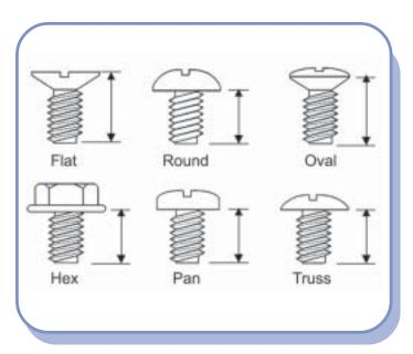
Figure 4.4–Screw Length Measurement
