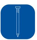
**structural bolt**, which connects wood to steel or wood to wood. Low-strength ASTM A307 bolts are commonly used in residential construction as opposed to high-strength ASTM A325 bolts, which are more common in commercial applications. Bolt diameters in residential construction generally range from 1/4 to 3/4 inch (6 to 13 mm), although 1/2- to 5/8-inch-diameter (13 to 16 mm) bolts are most common, particularly for connecting a 2x wood sill to grouted masonry or concrete.
