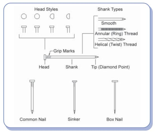
Figure 4.14–Elements of a Nail and Nail Types
