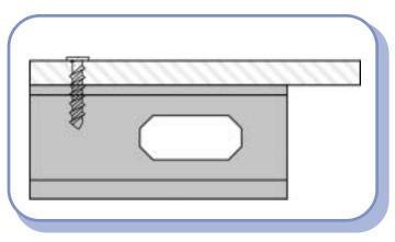
Figure 4.18–Wood Sheathing to Steel Connection
