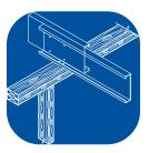
**Jack Stud.** A stud that does not span the full height of the wall and provides bearing for headers.
