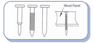
Figure 4.11–Pneumatically Driven Pins
