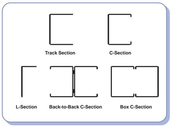
Figure 3.1–Typical Cold-Formed Steel Sections
