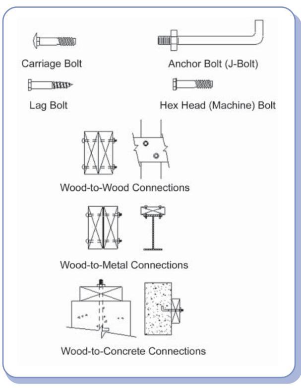
Figure 4.15–Bolt and Connection Types
