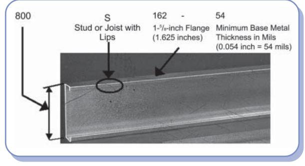
Figure 3.4–Standard Designation Illustration–Joist
