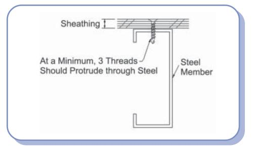
Figure 4.8–Fastening Sheathing to Steel
