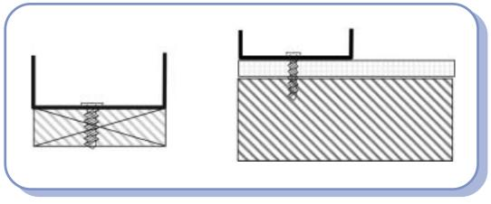
Figure 4.20–Steel to Wood Connection
