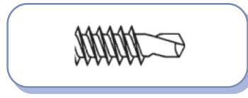
Figure 4.2–Self-Drilling Tapping Screw
