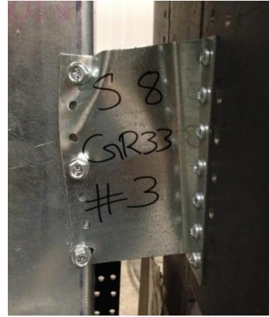
Figure 2.5: Test result of clip angle S8 #3
