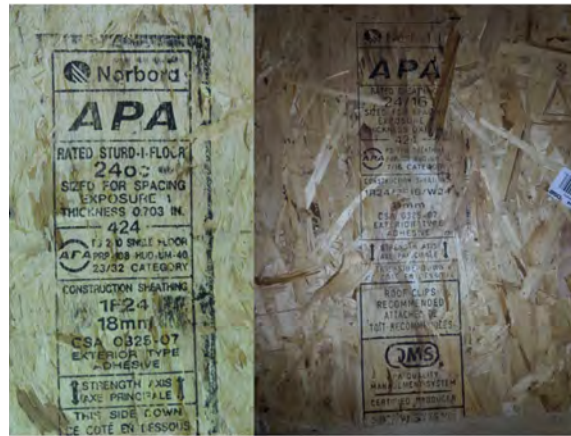
Figure 9: OSB panel grade stamps
