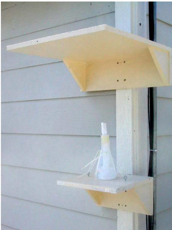
**Figure D.72: Chloride Candle and shield**
