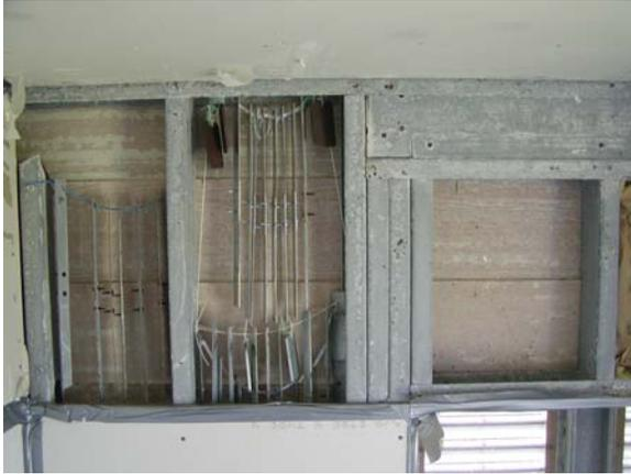
**Figure E.142: W wall – Lap siding w/o barrier**
