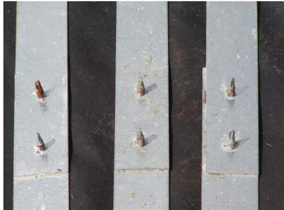
**Figure A.68: 7 Month exterior connection fasteners**
