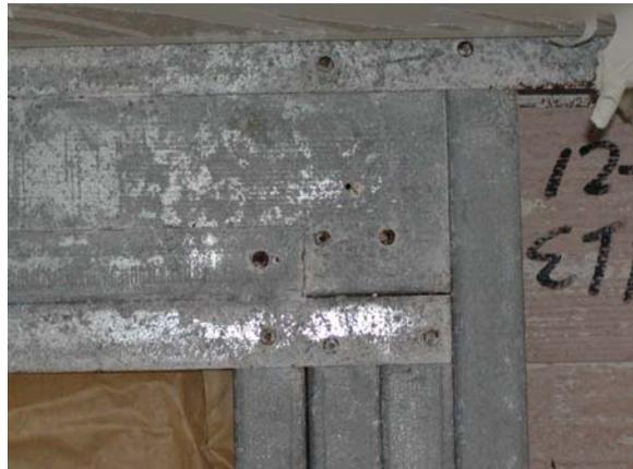
**Figure E.145: W wall header connection - right**
