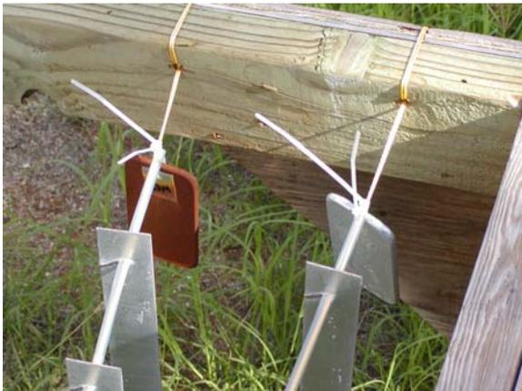
**Figure C.82: Location 5 – Steel and zinc coupons**
