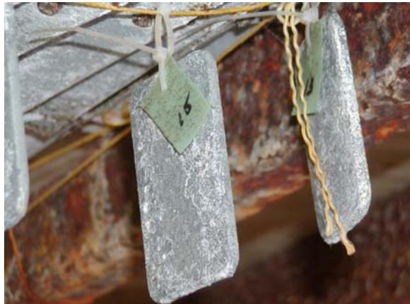
**Figure E.163: Open crawl space – zinc coupons**
