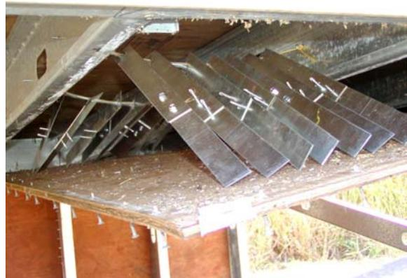
**Figure A.20: Covered crawl coupons – location 4**
