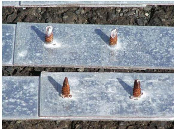
**Figure D.131: 7 Month exterior fasteners**
