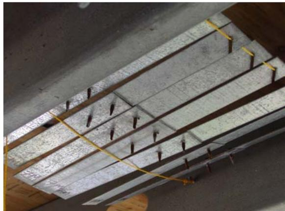
**Figure D.95: 7 Month exterior exposure specimens**
