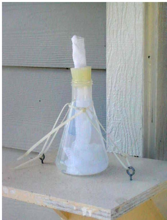
**Figure D.73: Chloride Candle**
