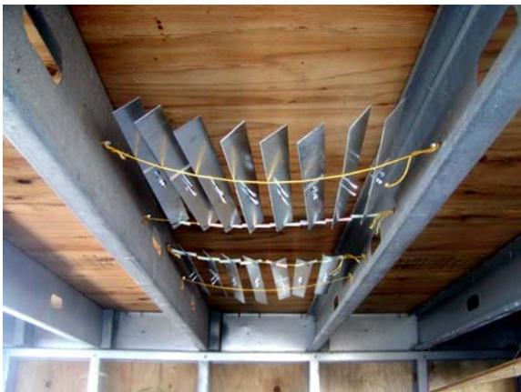
**Figure D.60: Test coupons in location 6 - exposed**
