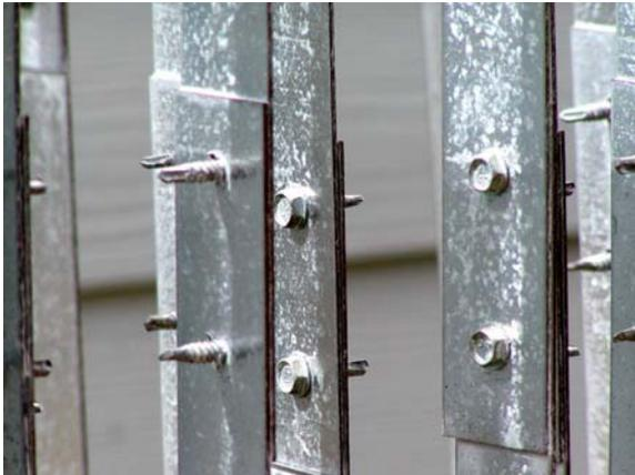
**Figure D.76: Close-up of 3 Month exposure**
