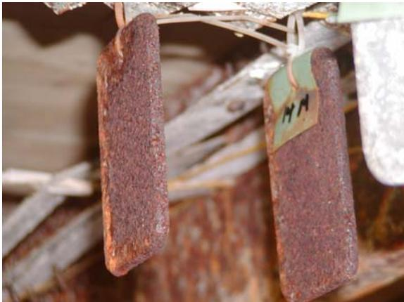
**Figure E.162: Open crawl space – steel coupons**
