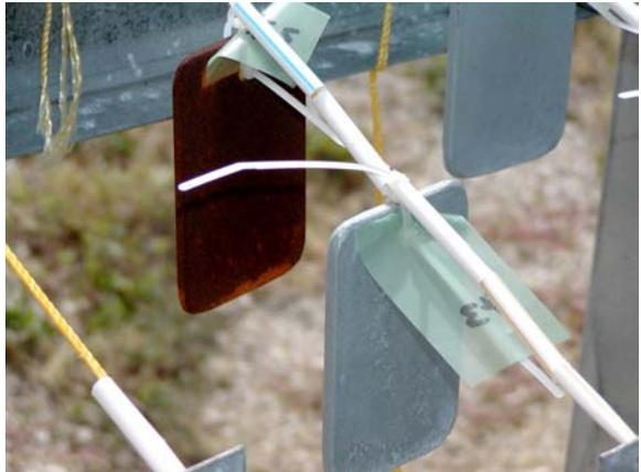
**Figure D.77: Steel and zinc coupons – 3 Months**
