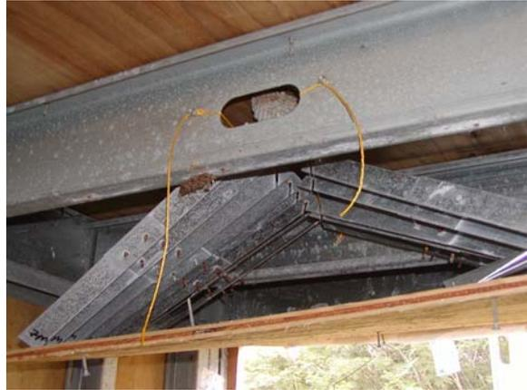
**Figure D.99: 7 Month exterior specimens added**
