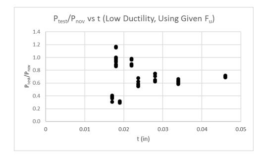
Figure 3.3 – Tested strength to nominal strength ratio versus thickness for low-ductility data (using given  $F_u$  Value)
