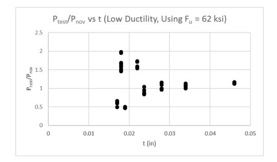
Figure 3.4 – Tested strength to nominal strength ratio versus thickness for low-ductility data (using  $F_u = 62$  ksi)
