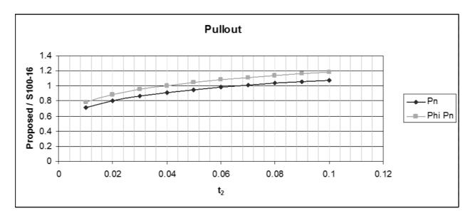
Figure 4.14 Effect of proposed adjustment factor upon pull-out strength
