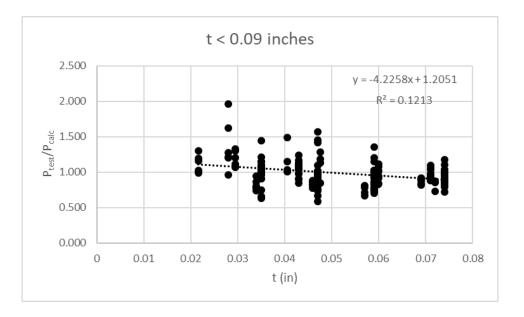
Figure 4.13 Adjusted  $P_{test}/P_{calc}$  versus t for t < 0.09 inches
