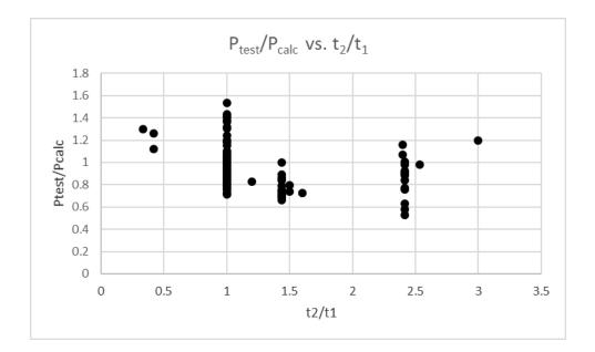
Figure 2.2 Effect of thickness ratio on low-ductility data
