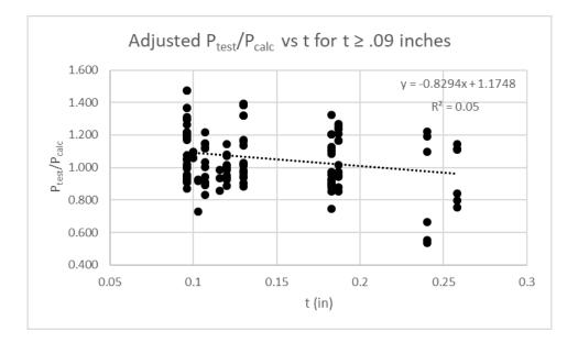
Figure 4.11 Adjusted  $P_{test}/P_{calc}$  versus t for  $t \ge 0.09$  inches
