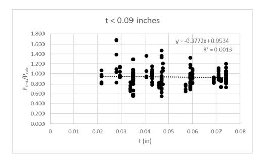
Figure 4.12 Original  $P_{test}/P_{calc}$  versus t for t < 0.09 inches
