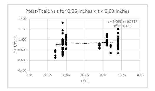
Figure 4.8 Original  $P_{test}/P_{calc}$  versus t for 0.05 inches < t < 0.09 inches
