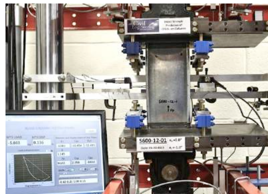
Specimen (S600-12-1) at post-peak stage (PP)
