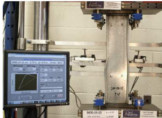
Specimen (S600-24-13) at post-peak stage (PP)
