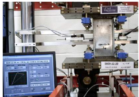
Specimen (S600-12-20) at post-peak stage (PP)
