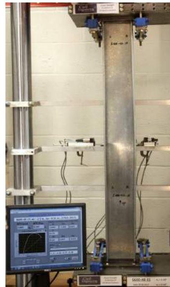
Specimen (S600-48-15) at post-peak stage (PP)
