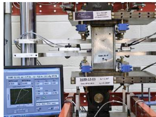
Specimen (S600-12-3) at post-peak stage (PP)
