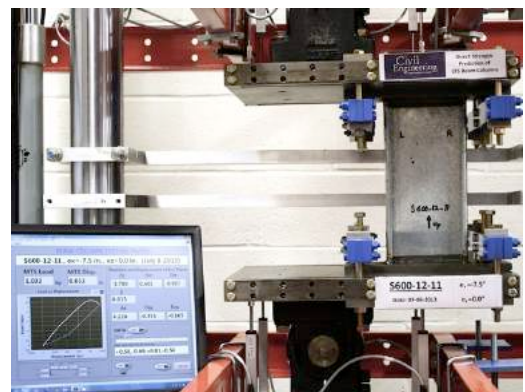
Specimen (S600-12-11) at post-peak stage (PP)
