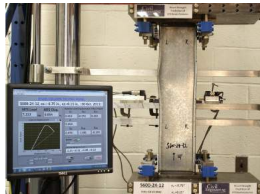
Specimen (S600-24-12) at post-peak stage (PP)
