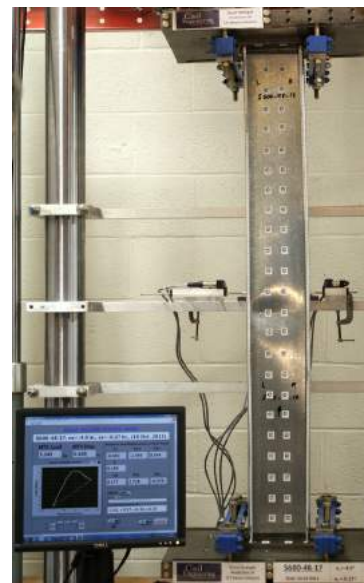
Specimen (S600-48-17) at post-peak stage (PP)
