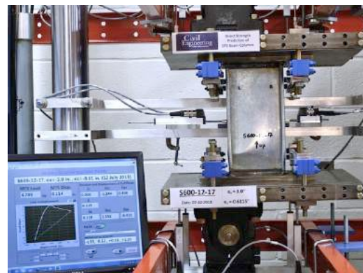
Specimen (S600-12-17) at post-peak stage (PP)
