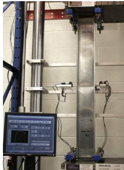
Specimen (S600-48-3) at post-peak stage (PP)
