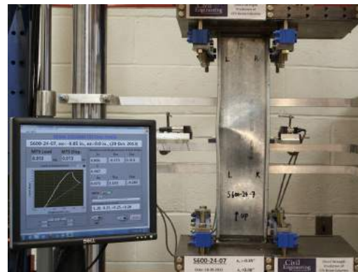
Specimen (S600-24-7) at post-peak stage (PP)
