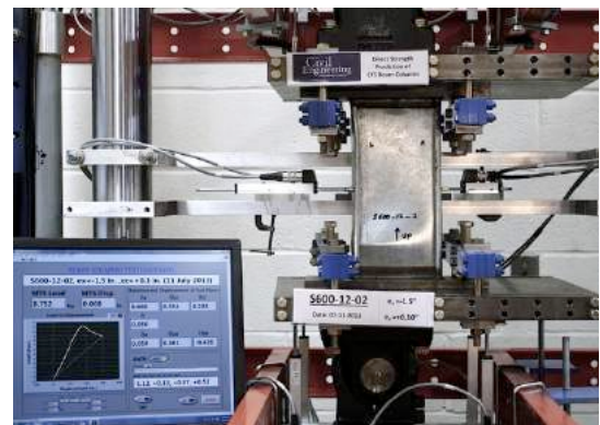
Specimen (S600-12-2) at post-peak stage (PP)
