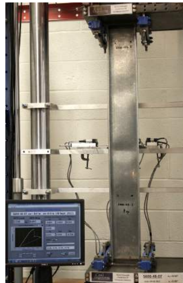
Specimen (S600-48-7) at post-peak stage (PP)
