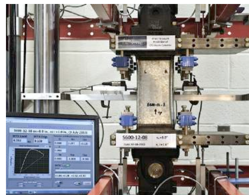
Specimen (S600-12-8) at post-peak stage (PP)
