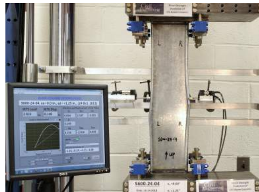
Specimen (S600-24-4) at post-peak stage (PP)
