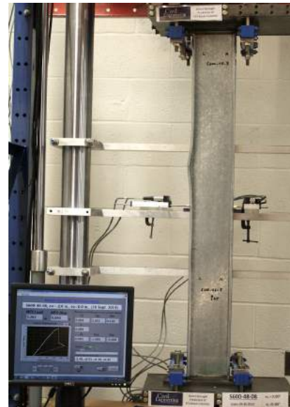
Specimen (S600-48-8) at post-peak stage (PP)
