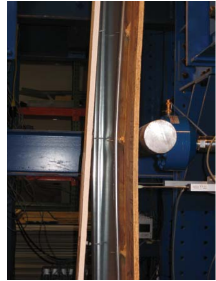
(c) GO specimen exhibiting pull-through (PT) failures on loaded OSB board
