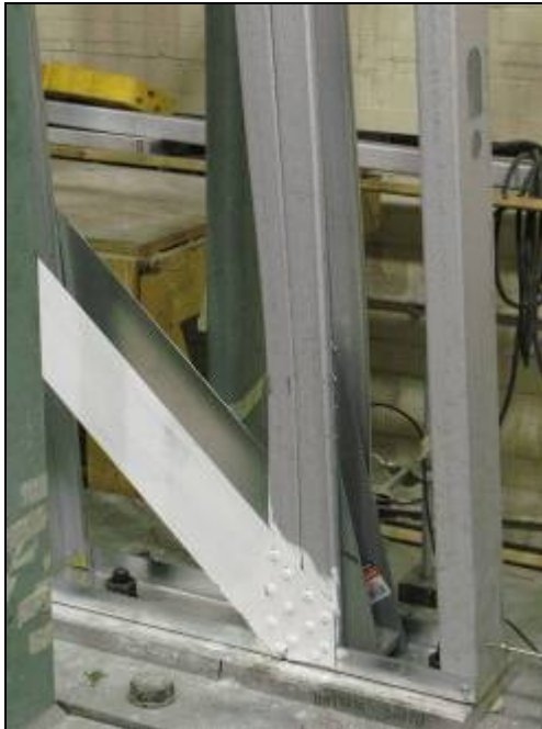
Figure 2.19 Corner detail of specimens 31 A-M and 35A-M
