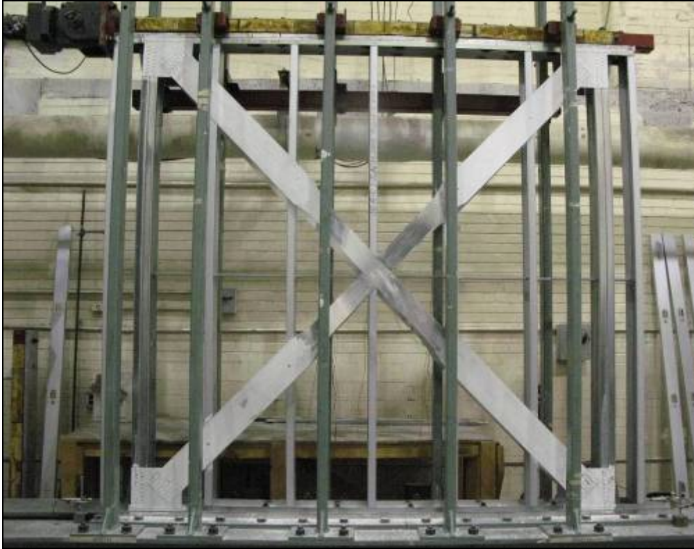
Figure 2.50 Test Specimen photographs showing elongated fuse section
