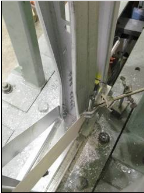
Figure 2.52 Distortional buckling of a chord stud of specimen 25A-M 1 (left) and net cross-section failure of a brace of specimen 25A-M 2 at 3.6% drift (right)
