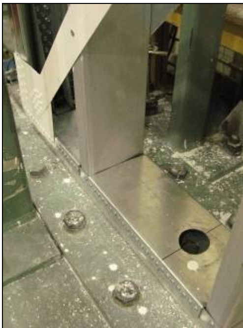
Figure 2.29 Holddown and track reinforcement detail of specimen 40 A-C
