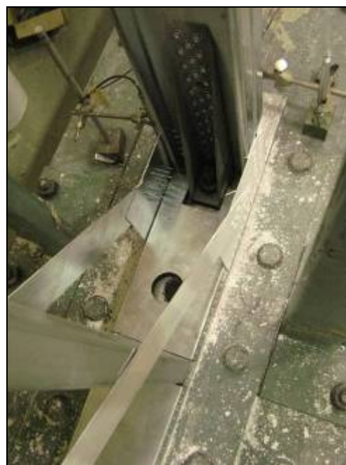
Figure 2.29 Holddown and track reinforcement detail of specimen 40 A-C
