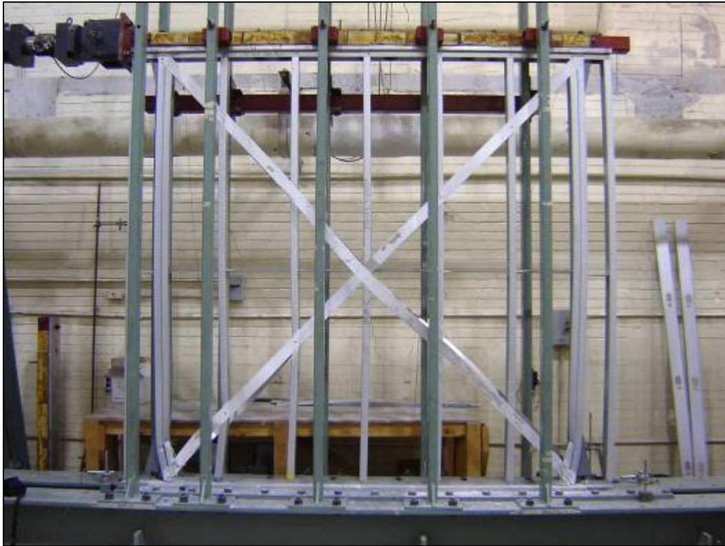
Figure 2.58 Bending of chord studs of specimen 36A-C
