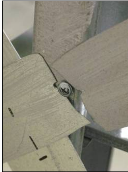
Figure 2.52 Distortional buckling of a chord stud of specimen 25A-M 1 (left) and net cross-section failure of a brace of specimen 25A-M 2 at 3.6% drift (right)
