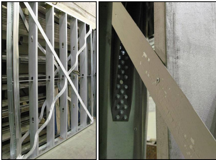
Figure 2.23: Medium walls showing brace yielding
