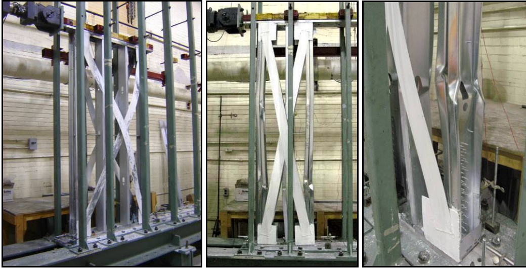
Figure 2.27: Post test specimen 24B-C (1220 x 2440mm); specimen 24C-C (610 x 2440mm)
