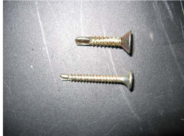
#10 and #6 screw, note head geometry, potentially important for pull-through resistance
