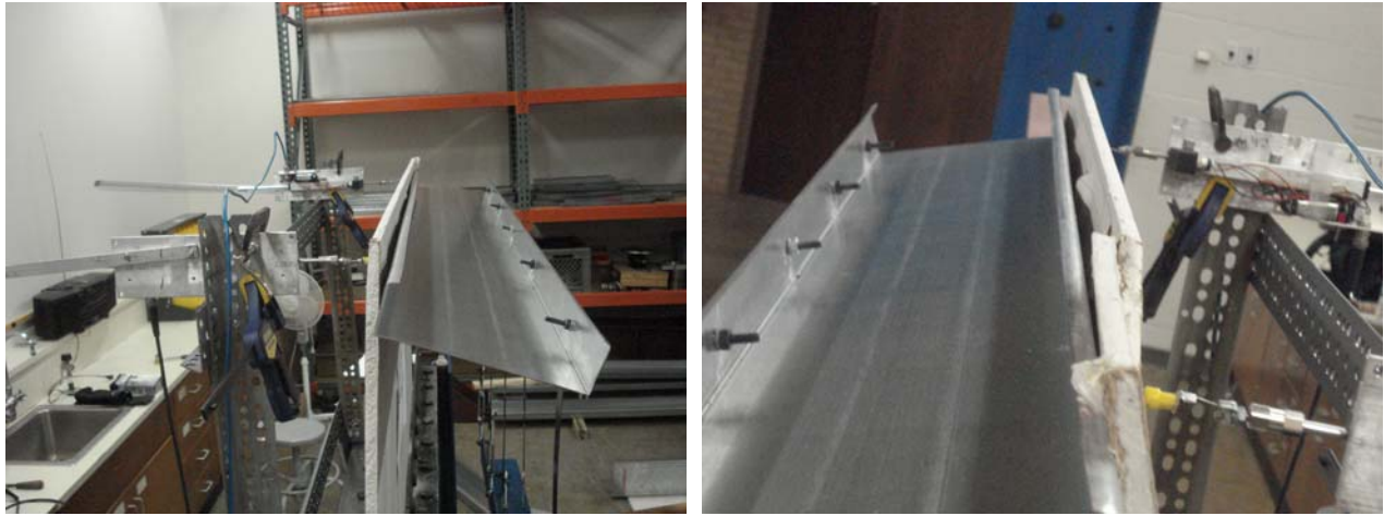
(a) large separation between joist and gypsum board with little bending in gypsum board shown for an 800S200-54 joist with gypsum board, L = 12 in., and #10 fasteners @ 12 in. (6-GYP-24-10-12-01, 6-800S200_54_33)
