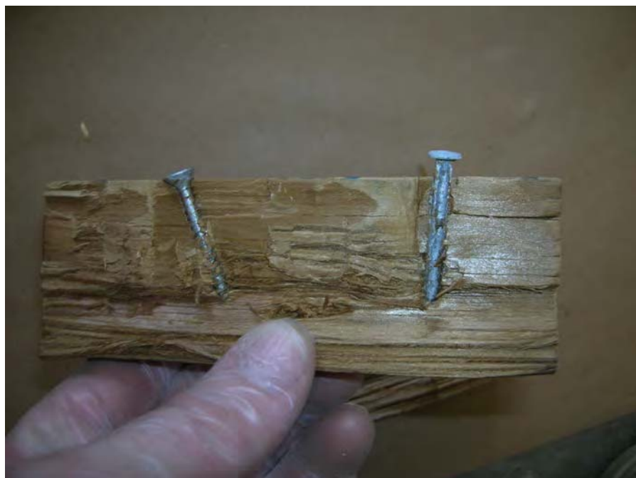
Photo 36 –Fastener Specimen After Testing – 30-Day
