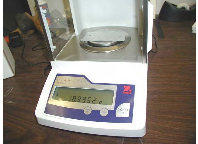
Photo 6 – Scale Used to Weigh Specimens
