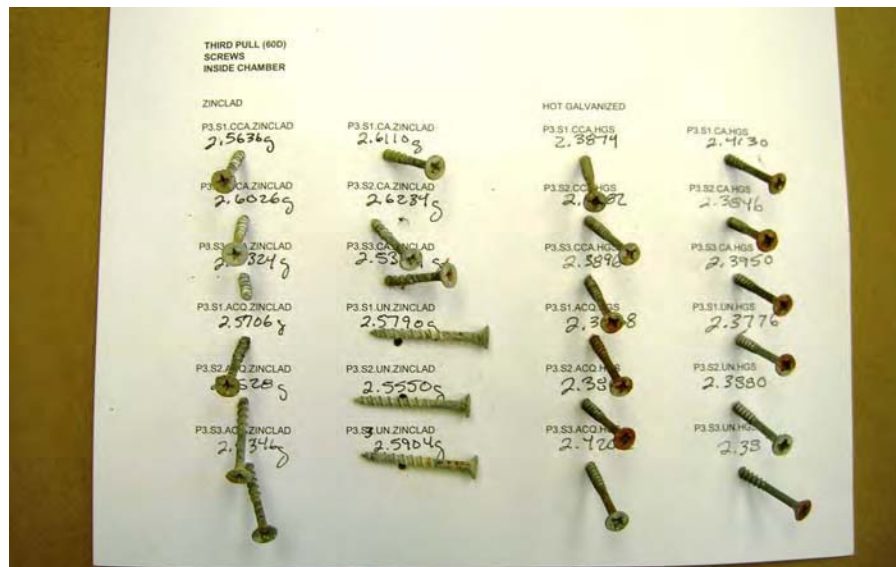
Photo 42 – Fastener Specimen After Testing – 90-Day
