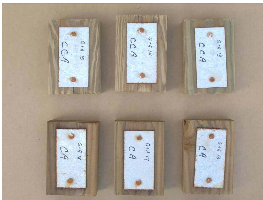
Photo 20 – Specimens Before Cleaning (30-Days)
