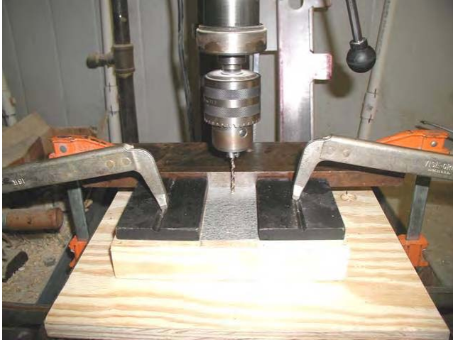
Photo 5 – Pre-Drilling Holes in Steel Coupons
