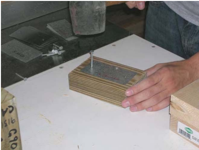
Photo 7 – Driving Nails Through Specimen
