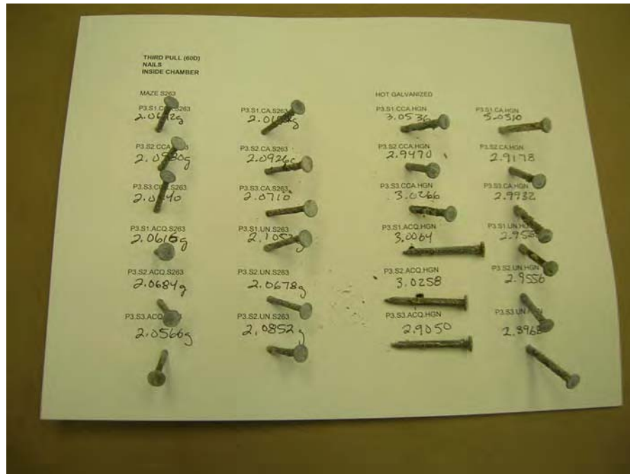
Photo 33 – Fastener Specimen After Testing – 15-Day
