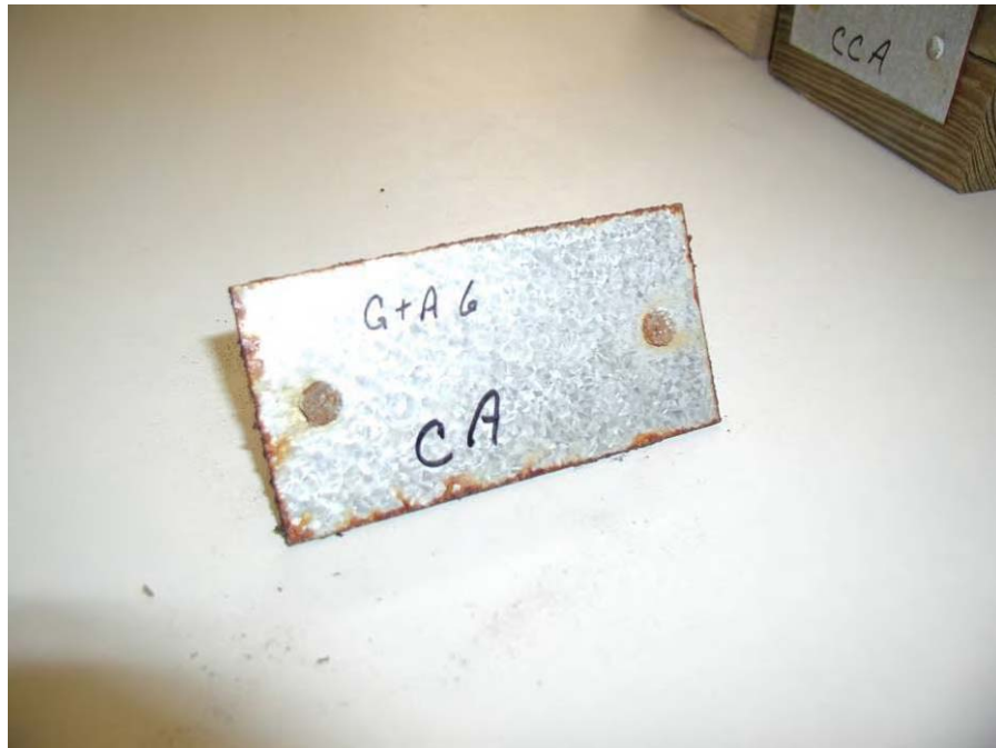
Photo 25 – Exposed Side of CA Treated Sample (30-Days)
