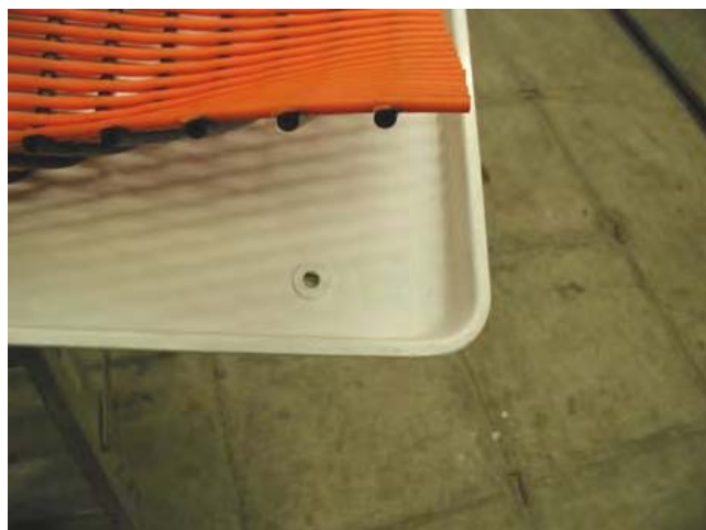
Photo 11 – Drainage for Each Rack
