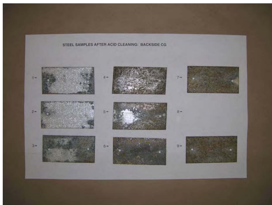
Photo 28 – Specimens After Cleaning (30-Days)
