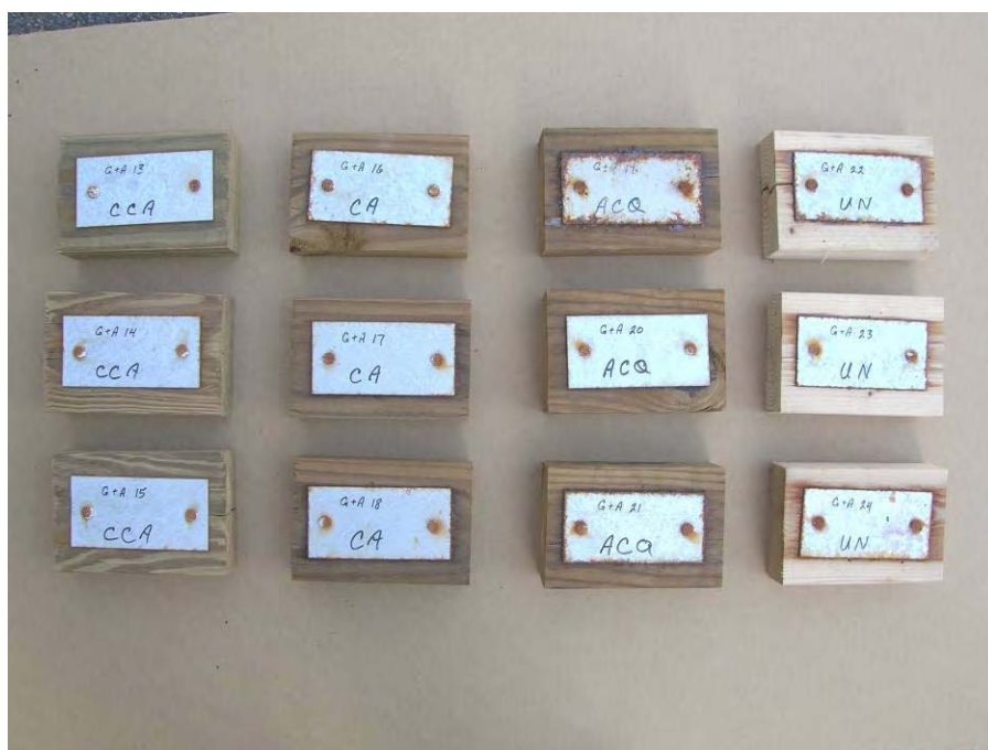
Photo 18 – Specimens Before Cleaning (30-Days)
