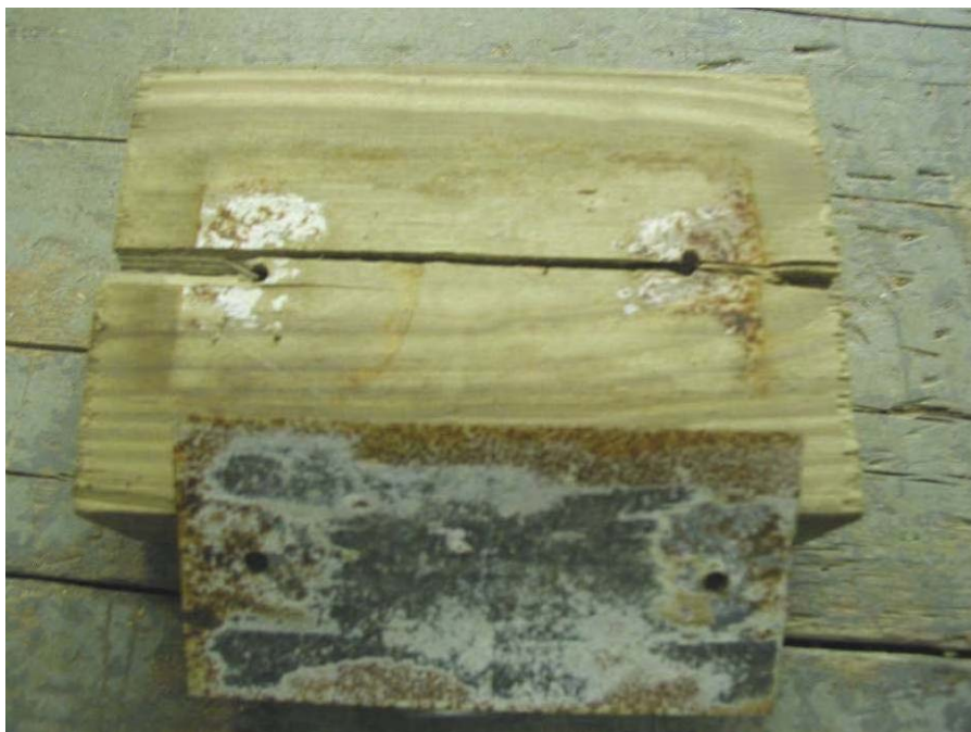
Photo 22 – Specimen in ACQ Treated Wood After 30-Days
