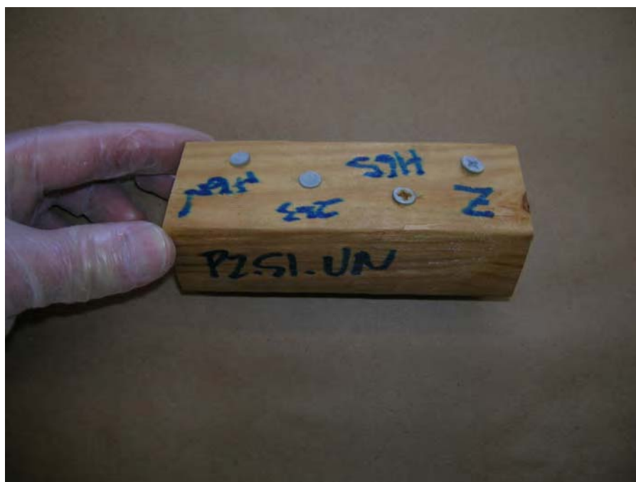
Photo 38 –Fastener Specimen After Testing – 30-Day
