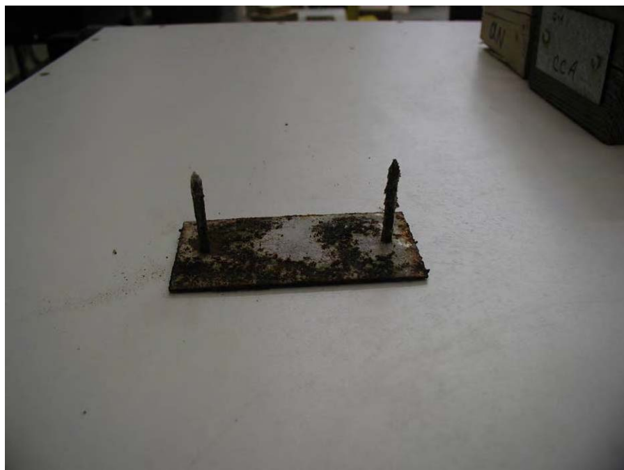
Photo 26 – Contact Side of CA Treated Sample (30-Days)
