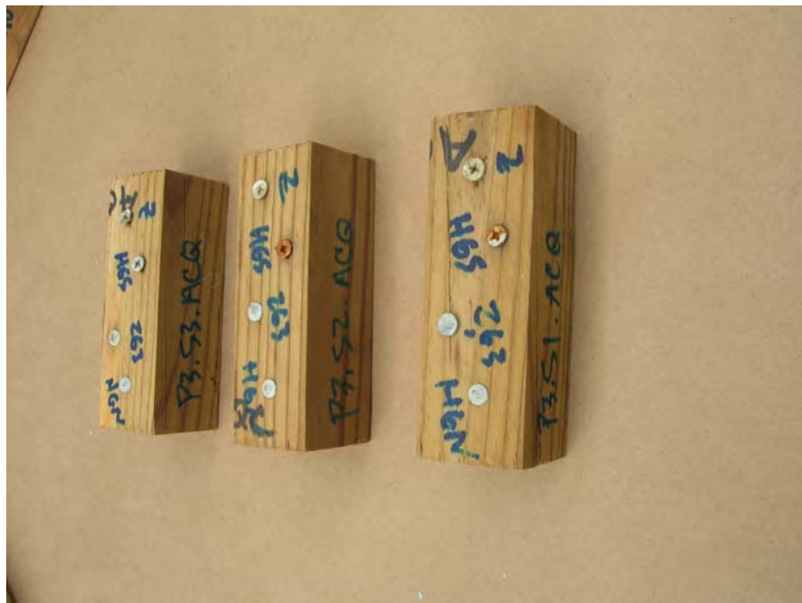
Photo 29 – Fastener Specimen After Testing – 15-Day
