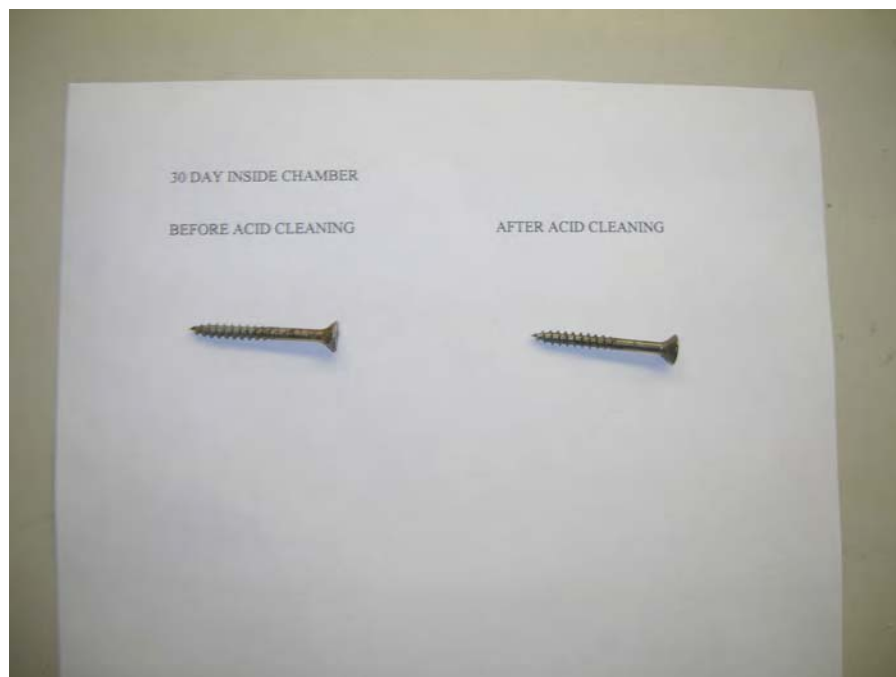
Photo 35 – Fastener Specimen After Testing – 30-Day
