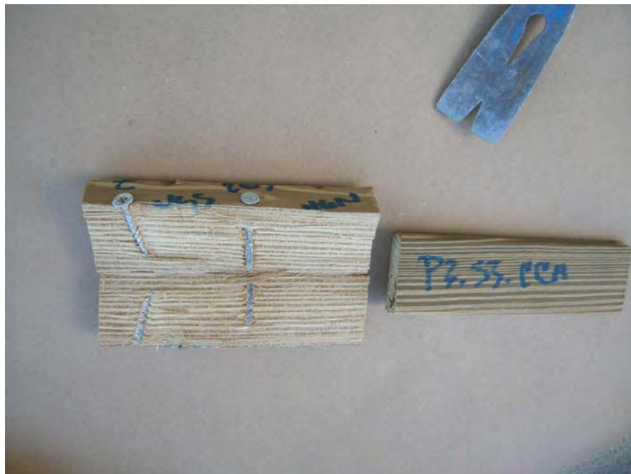
Photo 31 – Fastener Specimen After Testing – 15-Day
