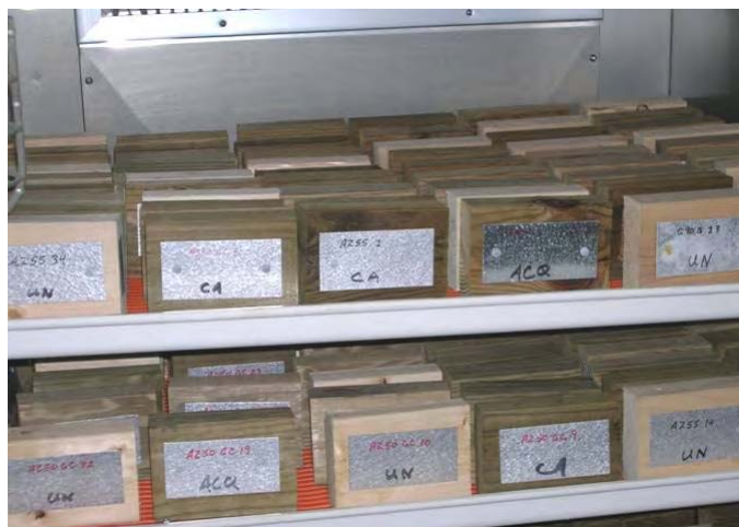
Photo 12 – Specimen inside Chamber
