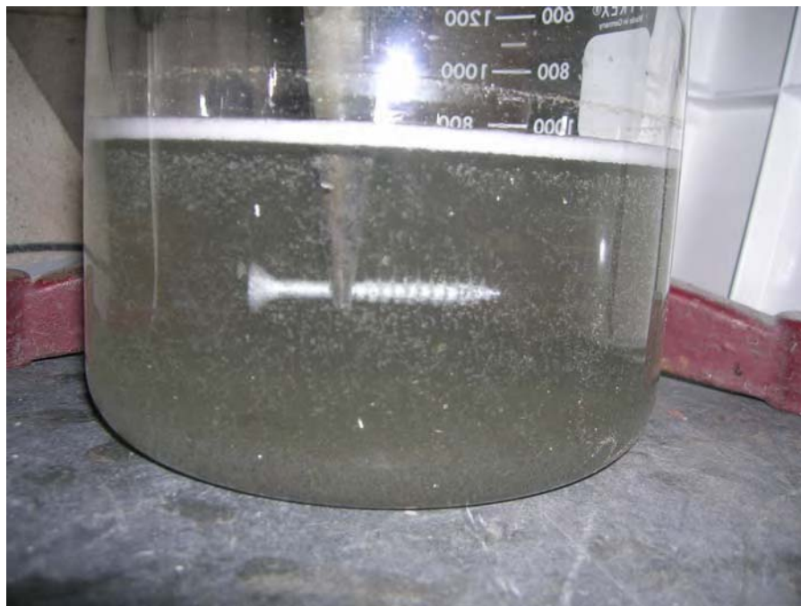
Photo 40 –Fastener Specimen During Cleaning – 30-Day
