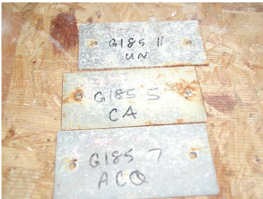
Photo 24 – ACQ, CA, & Untreated Retrieved Samples (30-Days)
