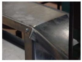
Figure 4.11-Buckling at Central Support
