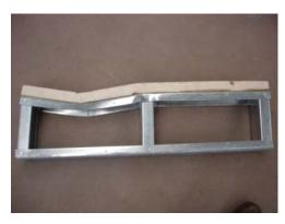
Figure 4.2 – Flexural failure of Specimen 1A16-18
