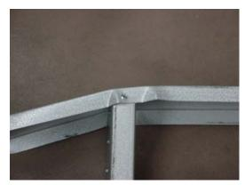
Figure 4.12-Failure of 18-ga. track
