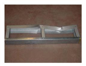
Figure 4.16 – Bearing Failures, Specimen Group E24-18
