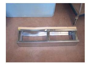
Figure 4.9 – Deformation of Specimen 2C16-16
