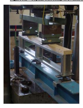
Figure 3.3 – Typical Test Setup Showing Placement of LSCs and Load Cells
