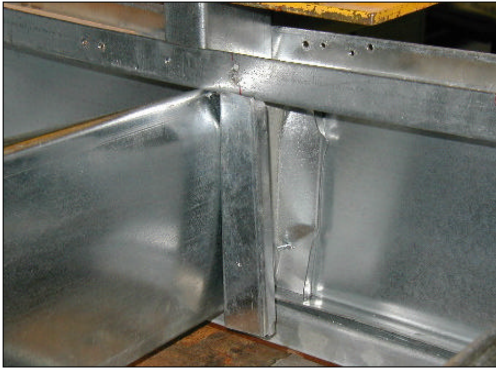
Figure 5.2: Photograph of a Stiffener Failure
