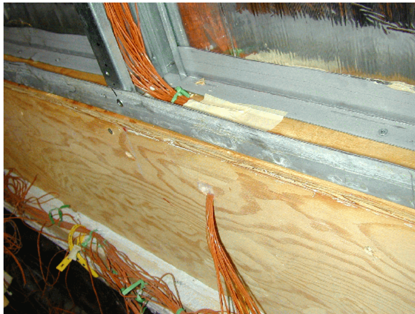
Figure 18 – Typical Split Track (Angles)
