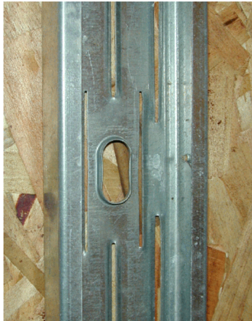
Figure 17 – Prototype of Slit Web Stud
