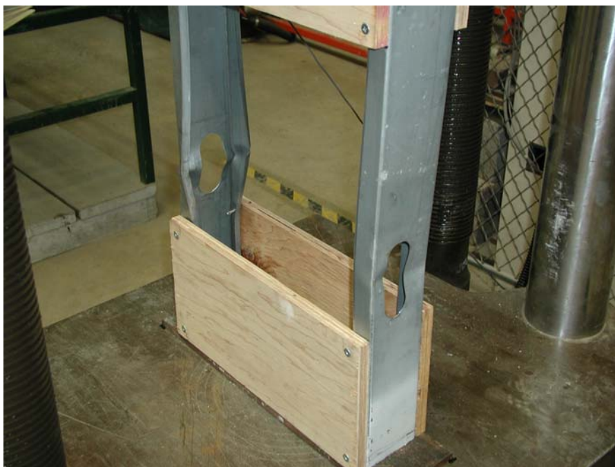
Solid Web Stud Failure Mode in Axial Tests
