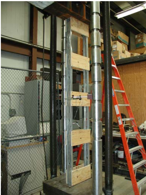
Slit-Web Stud Failure Mode in Axial Tests
