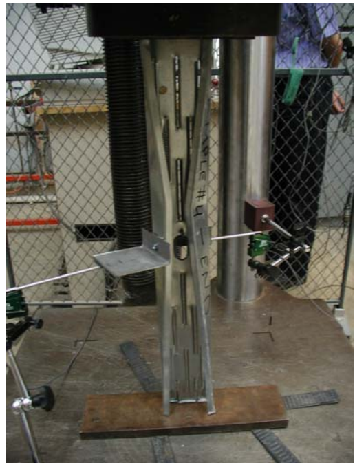
Slit-Web Stud Stub-Column Test Setup and Failure Mode
