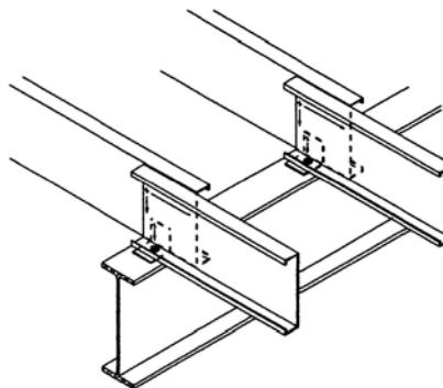
Solution: One continuous beam with two columns equally spaced is chosen. The top flange of the beam is to be braced at each joist (a positive connection is necessary between each joist and the beam). Provide a minimum of 1½ inches of bearing at the beam ends and 3½ inches of bearing at each column.
