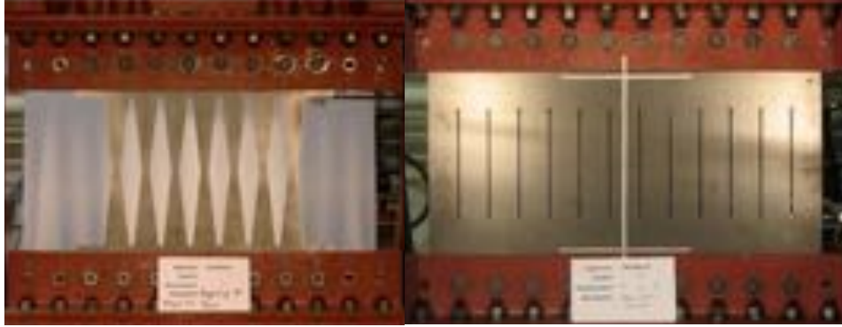
Figure 12 Early Energy Dissipation Devices Considered (a) Butterfly Fuse (b) Slit Fuse [from (Ma, 2010)]
