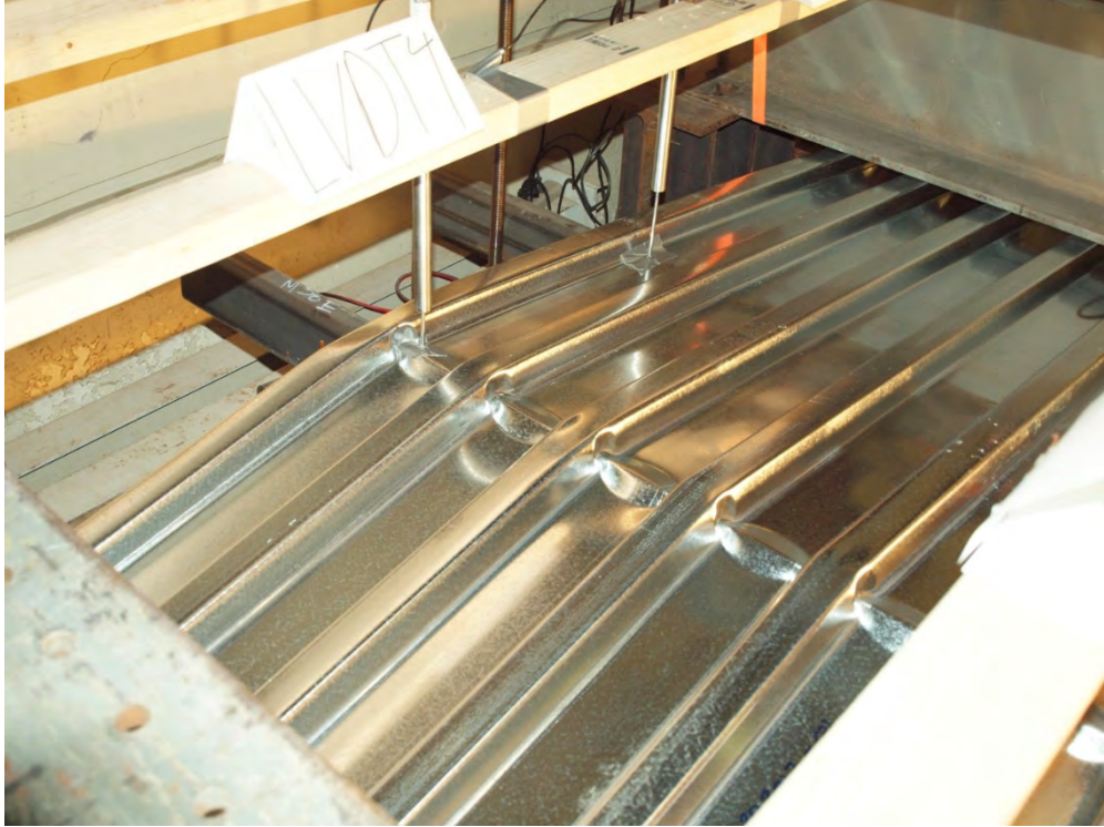
Figure 62: 20 Gage Deck Positive Bending - Final State.
