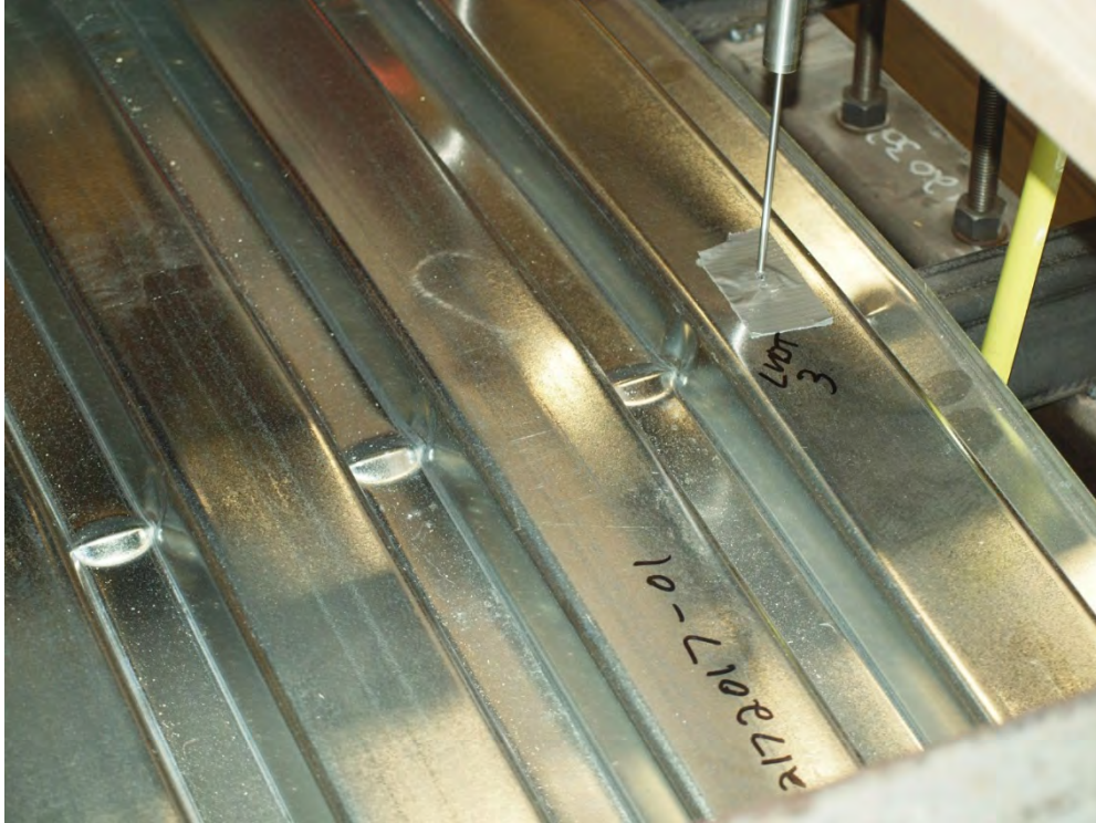
Figure 39: 18 Gage Deck Negative Bending - Initial Buckling.
