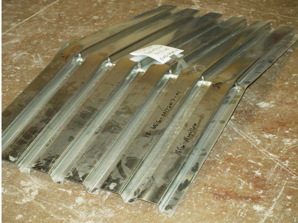
Figure 41: 18 Gage Deck Negative Bending - Final State.
