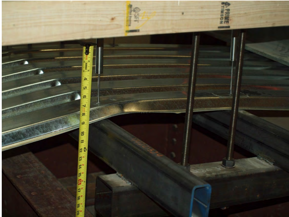
Figure 24: 16 Gage Deck Negative Bending - Final State.
