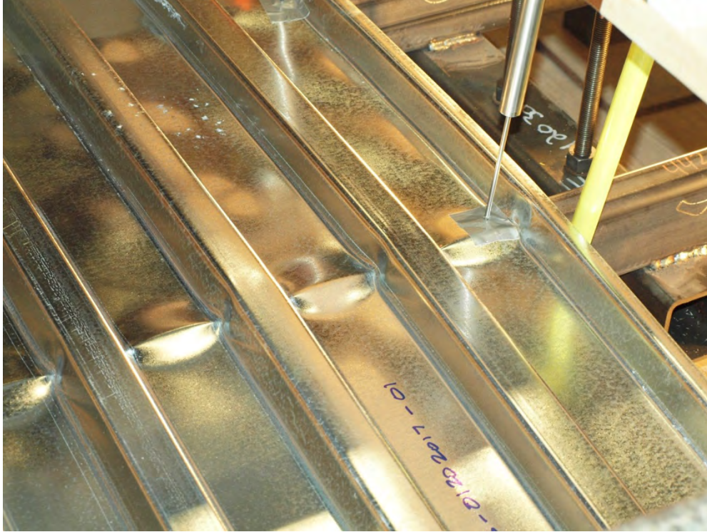
Figure 61: 20 Gage Deck Positive Bending - Further Buckling.
