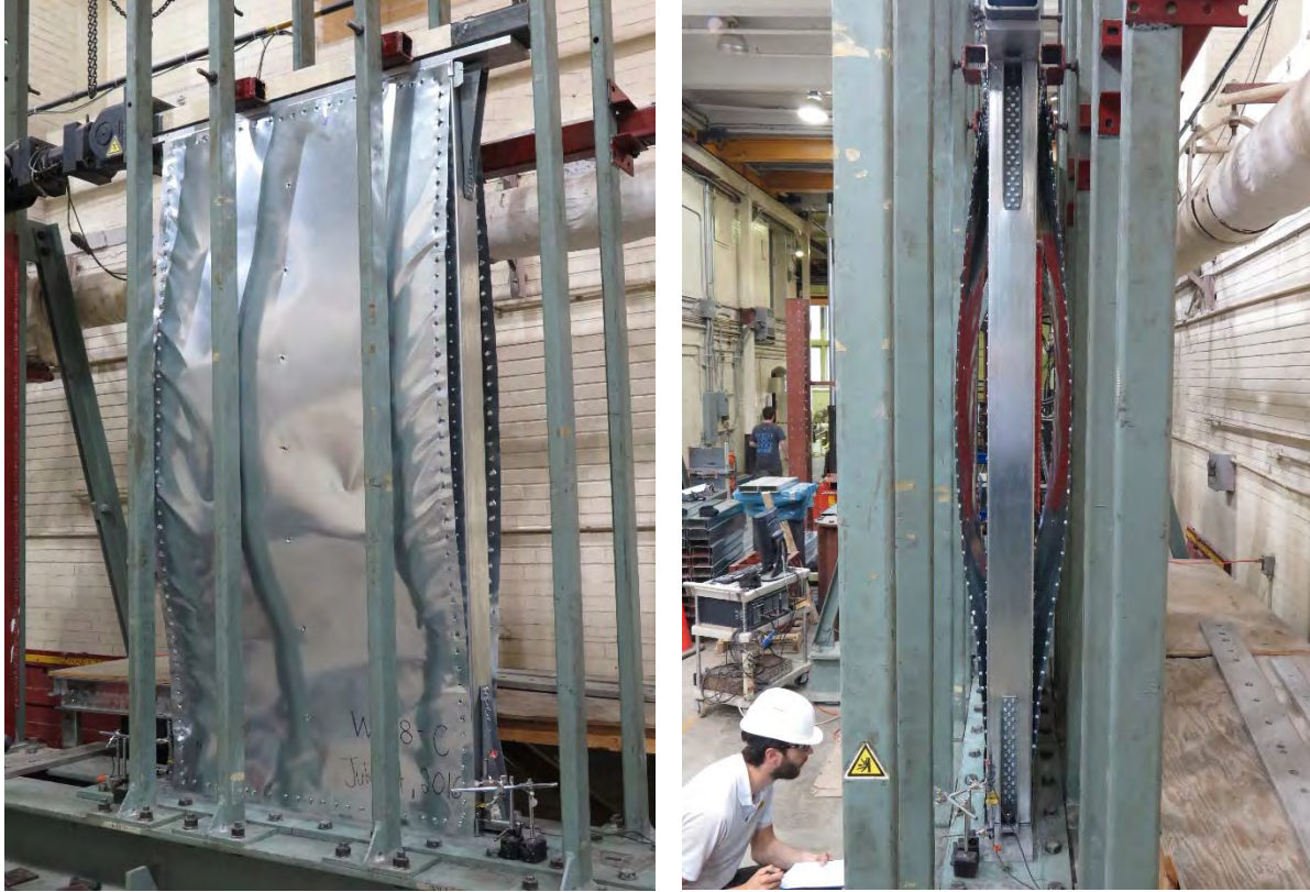
Figure 2.4: Sheathing detached from double-sheathed shear wall subjected to reversed cyclic loading.
