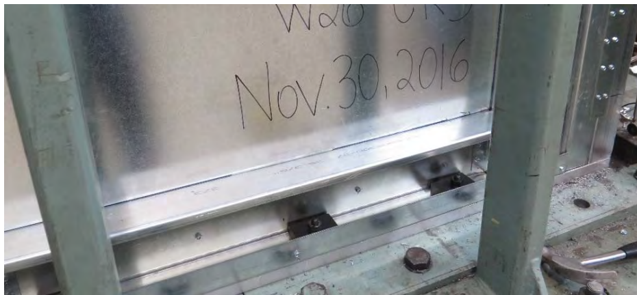
Figure 2.18: Placement of steel plates inside the flanges of the bottom horizontal framing member.
