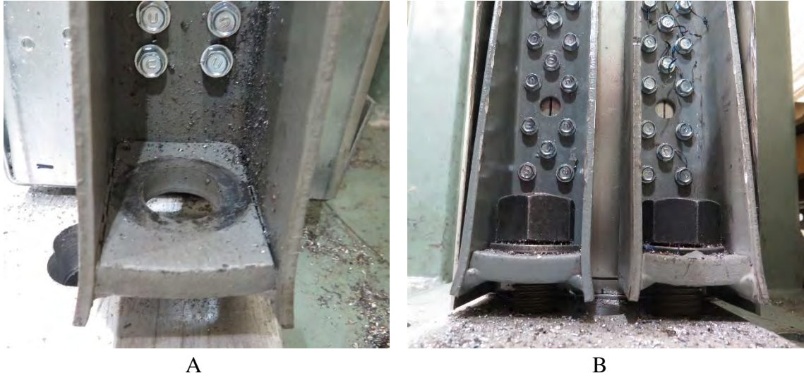
Figure 3.15: A) Single holdown plate damage. B) Double holdown plate damage.
