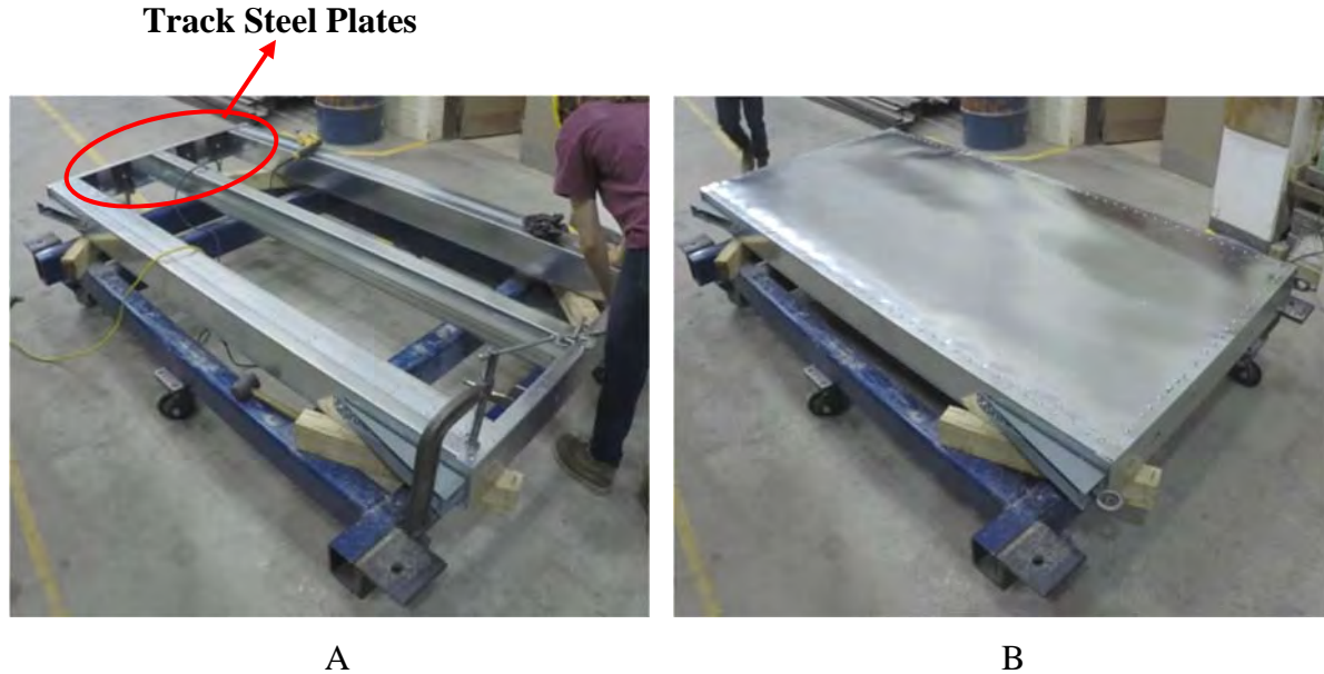
Figure 2.14: Assembly of a double-sheathed wall. A) Installation of field stud and track steel plates. B) Installed sheathing panel.
