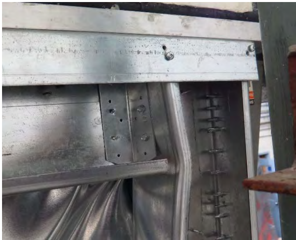
Figure 3.13: Chord stud flange damage at corners. A) Before installing stiffeners. B) After installing stiffeners.
