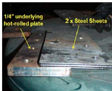
Figure 2.7: Perimeter shear configuration (Guenfoud, 2010).
