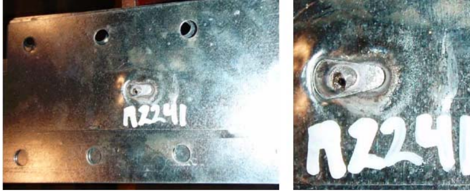
Figure 1.5: Sheet bearing failure mode (Guenfoud, 2010).
