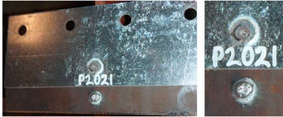
Figure 1.3: Shear weld failure (Guenfoud, 2010).
