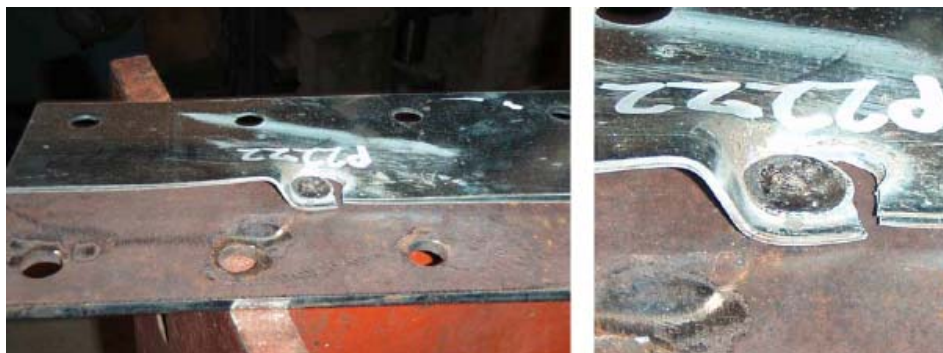
Figure 1.4: Sheet tearing failure mode (Guenfoud, 2010).
