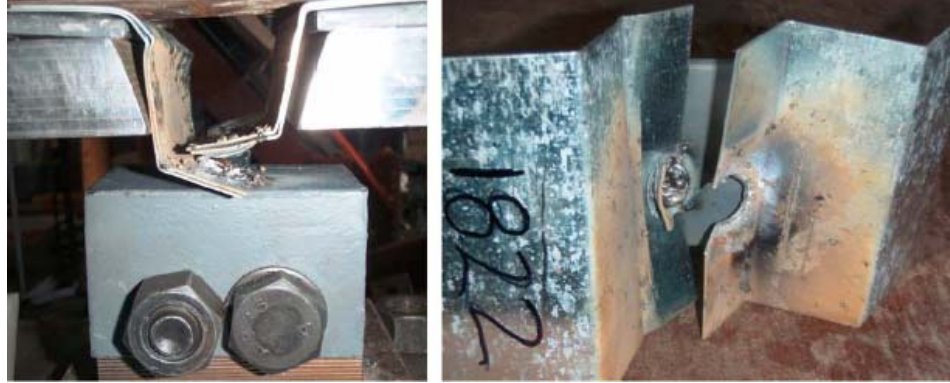
Figure 1.7: Tension sheet failure (Guenfoud, 2010).
