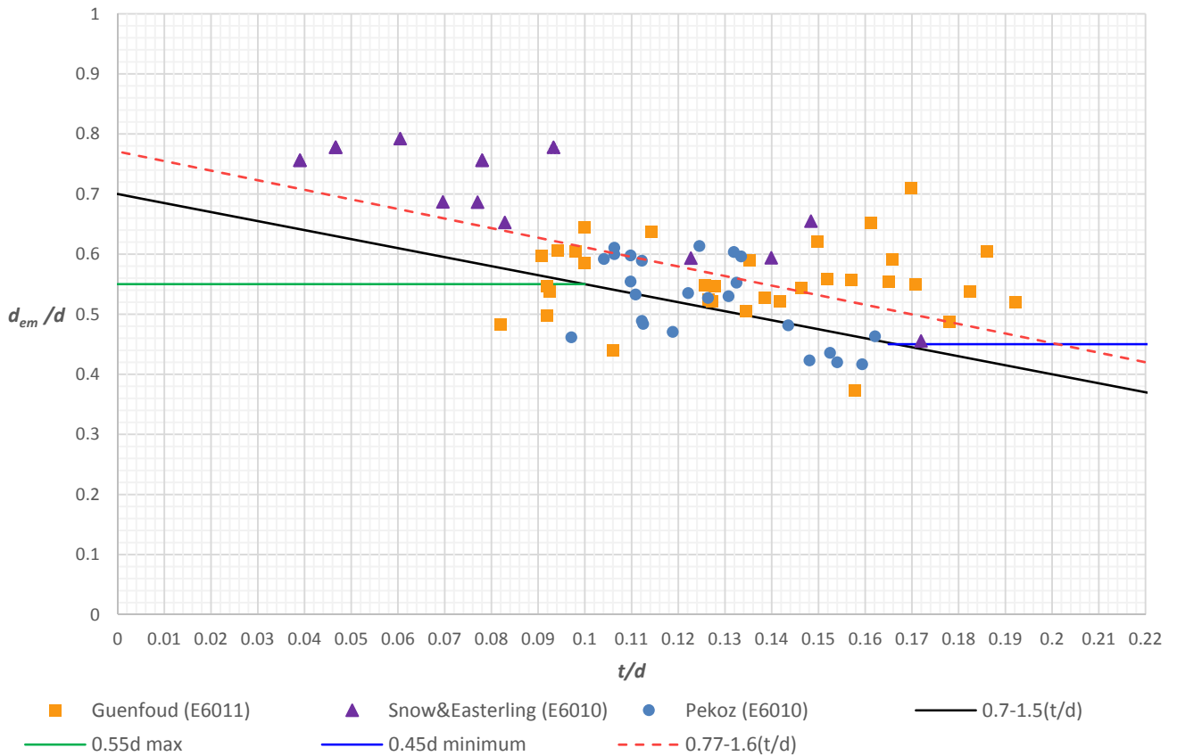
Figure 4.3: Evaluation of effective weld diameter with data from Pekoz, Snow and Easterling, and Guenfoud.
