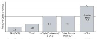
Note: The above data are based on accelerated testing per AWPA Standard E12-94, and may or may not have a relation to actual service life.
