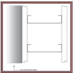
Figure 3. Wall with CI and no cavity Insulation
